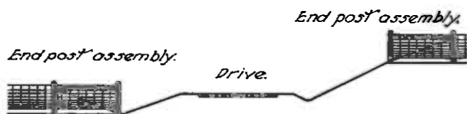
R/W FENCE TREATMENT AT DRIVES
